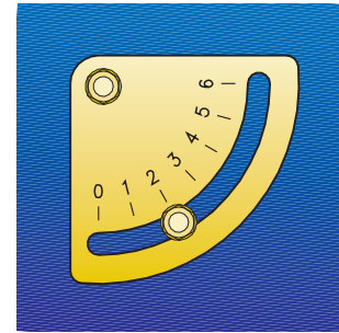
Example of fan air gate valve indexed selector of RL 28/1 burner
